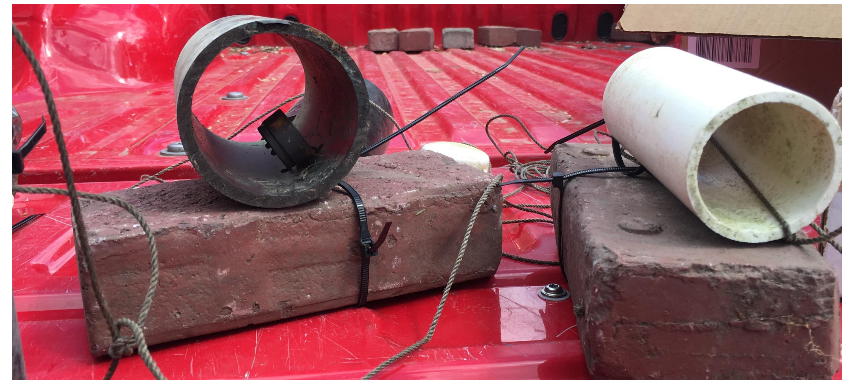
Figure 3. Hobo Pendant temperature loggers in a PVC shade were placed in the Spokane River to monitor water temperature.
